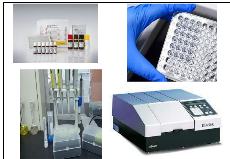
Figure 4: Determination of Aflatoxins B1 using A microplate Reader
