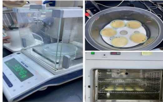
Figure 2: Measurement of moisture in samples
