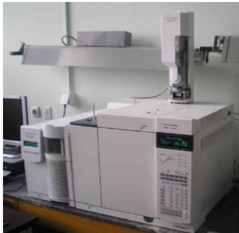
Picture 2. Hydrocarbons were analysed by GC–MS techniques. An Agilent 7890N gas chromatograph fitted with a HP5-MS capillary column (30 x 0.25 mm, 0.25 \mu m film; temperature range: 80 °C for 0 min; then 2 °C min -1 to 300 °C and held for 20 min) with helium as the carrier gas (flow rate 1 cm 3 min -1 ) was used.
