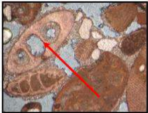
Plate4. Showing: Intragranular Porosity
